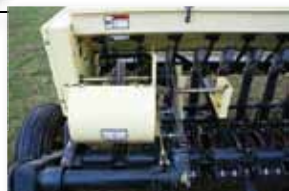
Gear Reduction Assembly To allow quick change and exact seed delivery calibrations.
